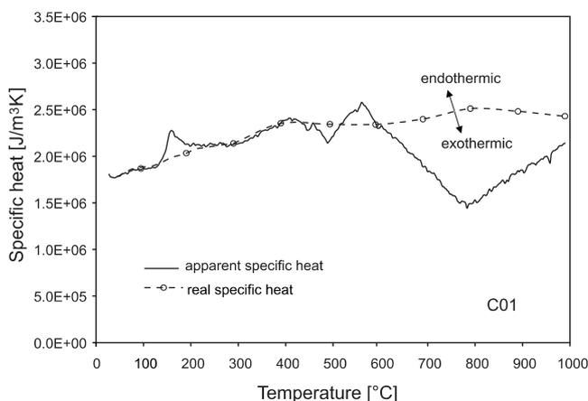
Fig. 5. Apparent and real specific heat of coking coal C04 and thermal coal C01
