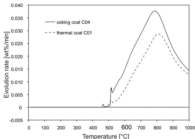
600 mass spectrometer and is shown in Figure 6. The hydrogen release in case of C04 was more pronounced reflected in the higher exothermic reaction. The contraction was also observed during the optical analysis of the two samples with higher effect in the case of coal C04.
