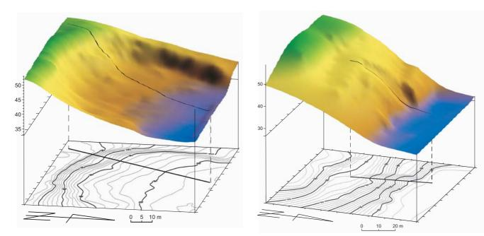
Fig. 5. Digital model and contour map of landslide surface according to detailed geodetic measurements (Bartoszyce area)
