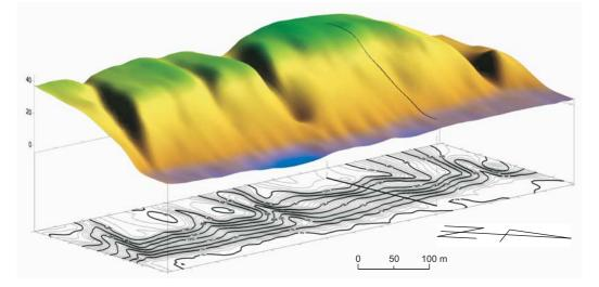
Fig. 4. Digital model and contour map of landslide surface according to detailed geodetic measurements (Chlapowo area)
