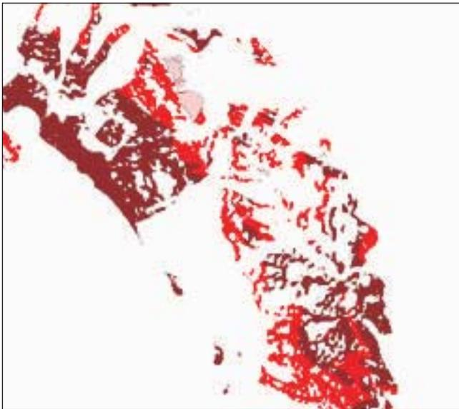
**Fig. 10. Intersection of landslipped areas with a map showing slope thresholds and material brittleness**
