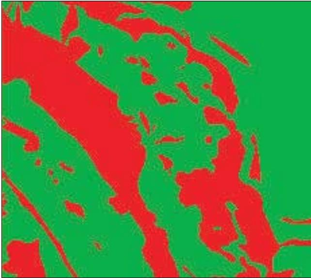
**Fig. 9. Non-brittle soil or hard rock (green) or brittle soil (red)**
