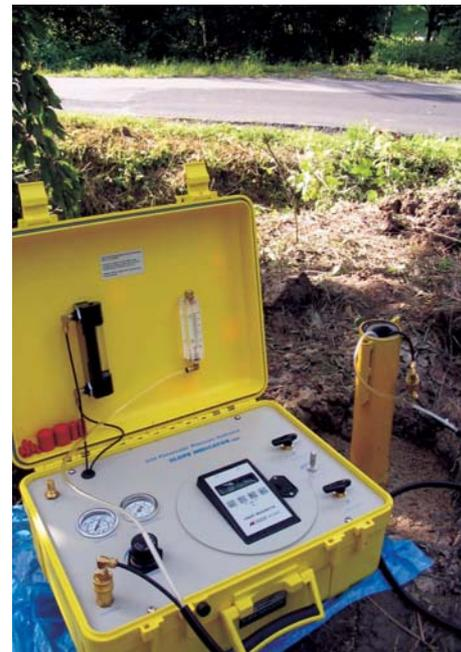
Fig. 18. Pore pressure measuring equipment
