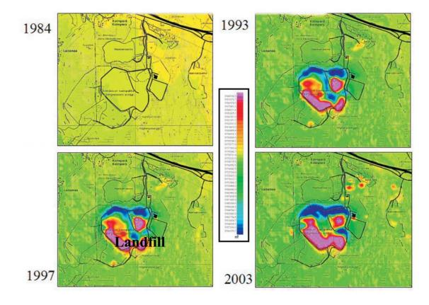
Fig. 3. The airborne total magnetic field maps from the Ämmässuo landfill
