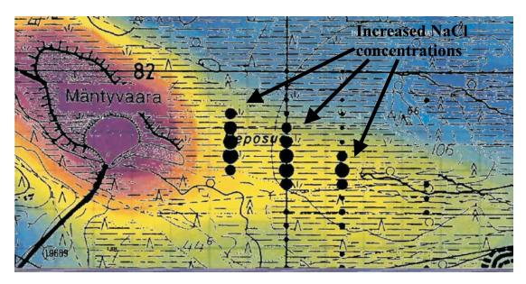
Fig. 5. The airborne electromagnetic out-of-phase component map from the Mäntyvaara landfill
