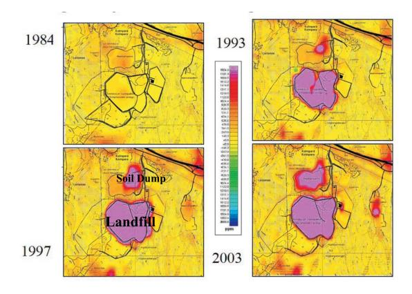
Fig. 4. The airborne electromagnetic out-of-phase component maps from the Ämmässuo landfill Purple colour indicates a strong electrical conductivity
